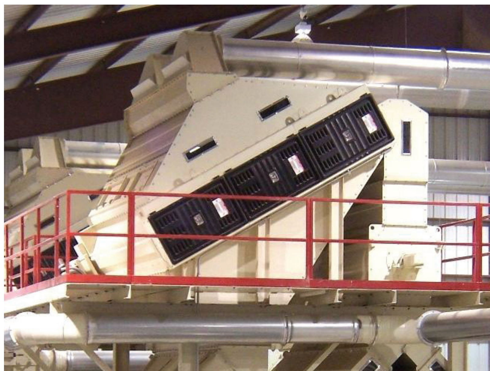
9-Cylinder Inclined Hot Air Cleaner (shown with dual Front-Entry Splatter-Back Inlets)
