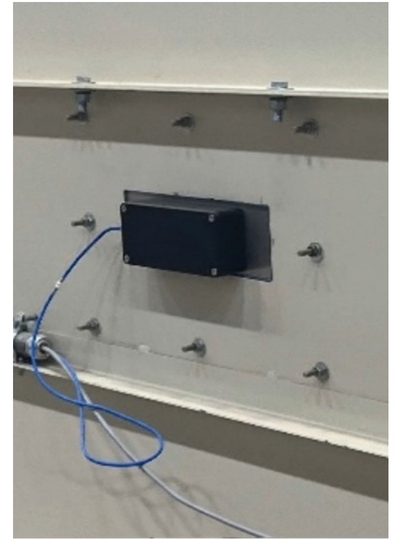
Moisture Sensor (left) inside Storage Hopper and Rear View of Moisture Sensor (right) on Overflow Hopper
