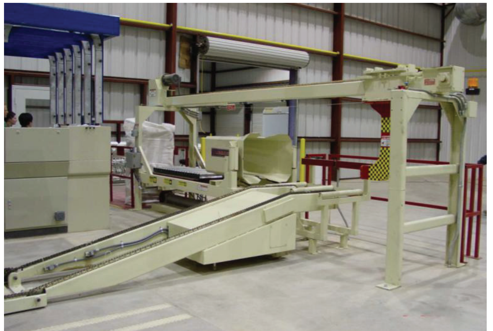
Bale Handling System for up-packing Press
