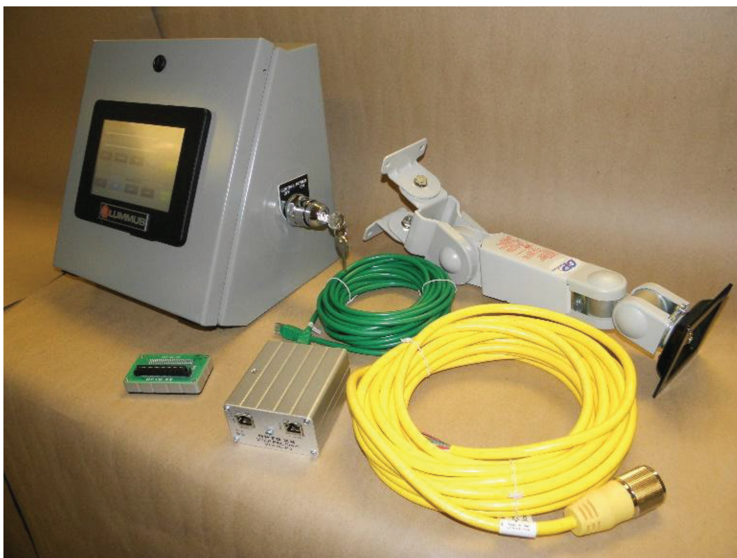
DGC 2020 Gin/Feeder Controls Operator Interface Conversion
